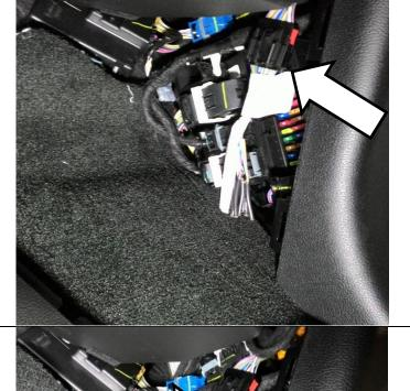
Plug in the 2017-2022 BD High Idle wiring harness to this connector.
