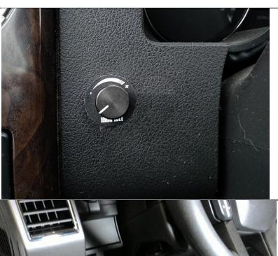
If mounting in the knee bolster, be aware of the reinforcement plate behind the bolster which will limit the available spaces to mount the switch.
