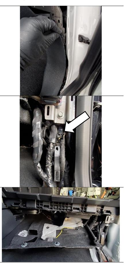
The pigtail location has been found to vary from truck to truck. Shown here is the most hidden and inaccessible spot. The metal bracket that held the plastic panels can be used as a reference point.
